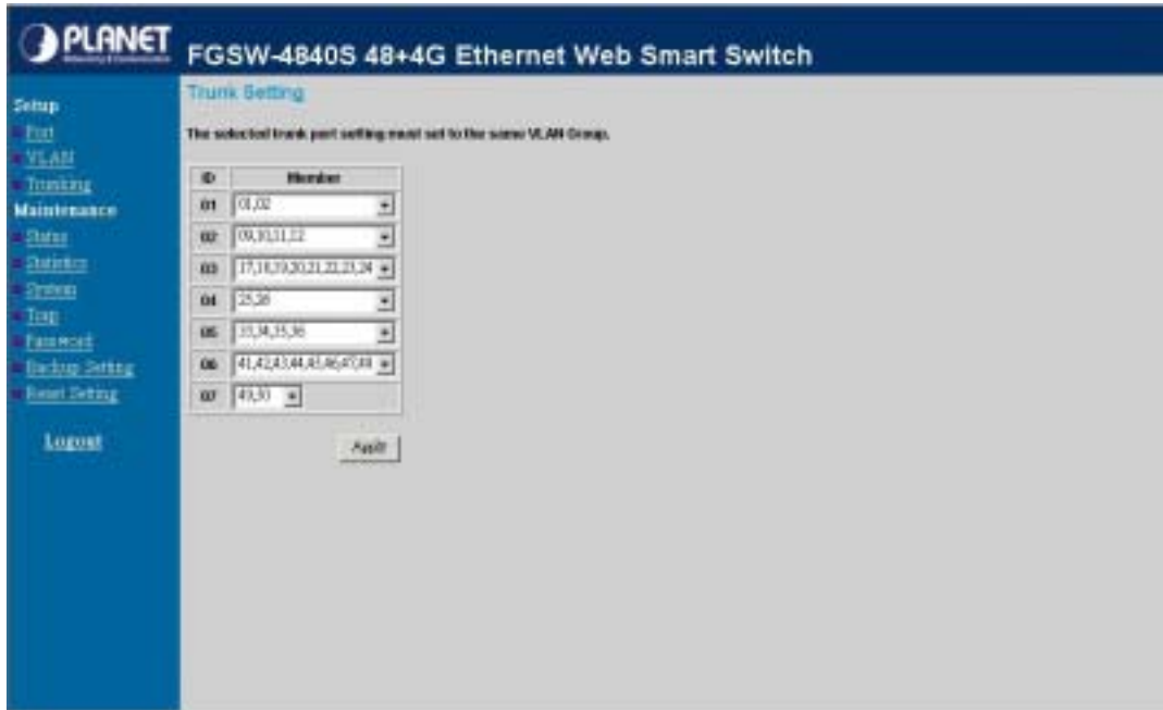
Figure 3-35 Trunking Setting screen
